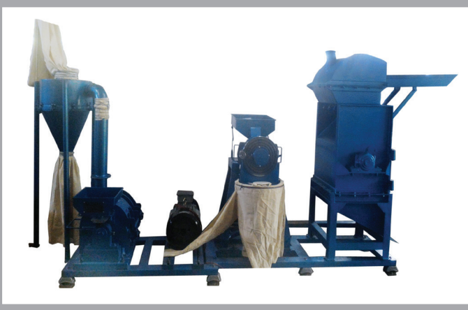
Powdering System - 3 in 1 Arrangement
